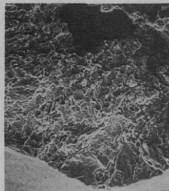
Figure 6. Cross-section with cavity from Mg-HD-prills (50 ×)
