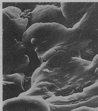
Figure 12. Detail of cross-section from Al-LD-prills (500 X)
