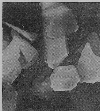
Figure 26. The SiO_2 -particles used (5000 ×)
