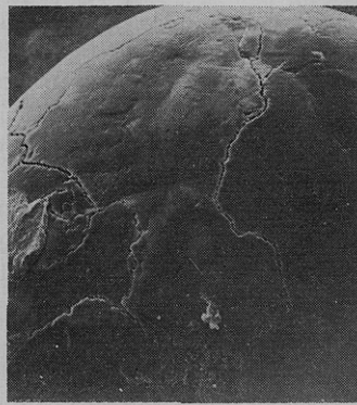
Figure 5. Surface from Mg-HD-prills (65 ×)
